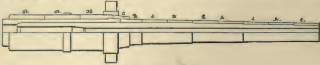
Naval 8-in. Breech-Loading Rifle.
